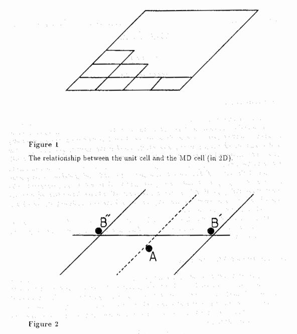
A problematic arrangement of ions in the proposed periodic boundary scheme (a 2D analogy). Ion A is near the centre line of the cell. The scheme will select the image B' in preference to B", which is actually the nearer of the two images. The use of an appropriate spherical cutoff removes this difficulty (see text).
