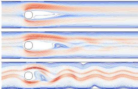
Seeing how obstacles affect flows of liquids and gases can be important. For example, wind flowing past a car aerial can make it vibrate, while strong winds past a power station cooling tower might apply stress and even cause it to collapse! More Commonly used in Engineering or Physics than Chemistry.
