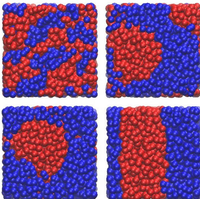
Observation shows that if you try to mix together two liquids that do not tend to mix, they will separate out. The interfacial tension between two liquids gives an idea of how much force they will apply to each other and how quickly they will separate.
